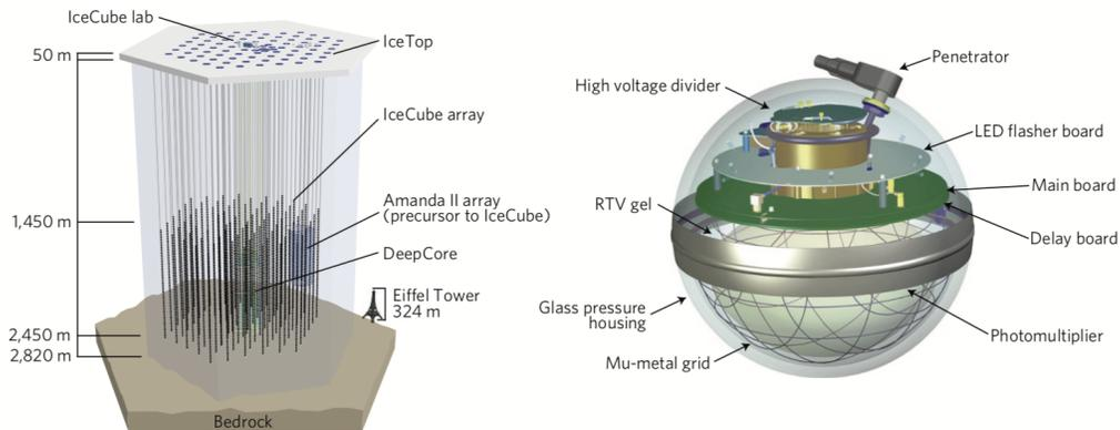
Figure 1: Left: IceCube observatory. Right: digital optical module
